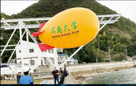
Photo 1: Capturing water surface images using a balloon for seagrass bed mapping
